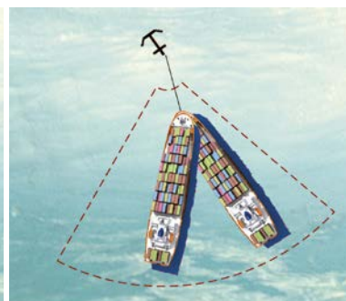
Anchor control mode Monitoring of the anchorage and automatic control of stern thrusters to keep the vessel on its heading and position.
