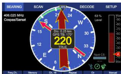
When MOB function is activated, the pink indicator shows the direction to the MOB position. The distance is indicated in the window.
