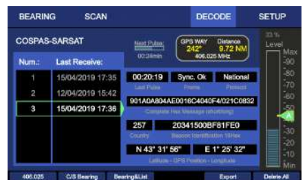
COSPAS-SARSAT decode page with list of all beacon information including indication to the GPS-Position (distance and direction)
