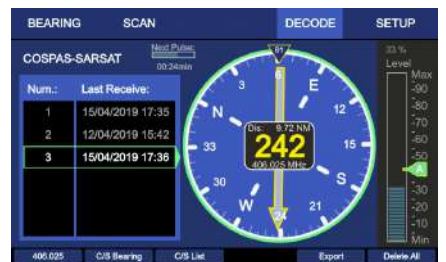
Decode page with direction and distance indication to COSPAS-SARSAT GPS-Position and list of reception history
