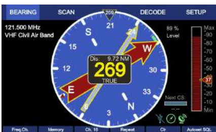
Standard bearing display with additional COSPAS-SARSAT GPS-direction indicator (indications can be different)
