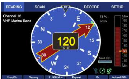
Standard bearing display shows bearing (true/magnetic or relative); signal level strength; working frequency or channel; heading status
